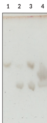
Lane 1: Lactose (control) Lane 2: Galactose (control) Lane 3: Negative control (no enzyme control) Lane 4: Reaction mixture with enzyme
