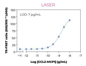
Figure 3 Typical nonlinear human CCL2/MCP-1 standard curves in Assay Buffer 1. Left: lamp excitation, Right: laser excitation. Data represent the mean ± standard deviation of triplicate measurements (3 wells) for each standard. The data was generated using a low-volume 384-well white plate read on the EnVision® equipped with TR-FRET option.
