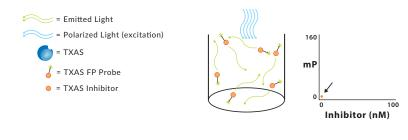
Large fluorescent molecules do not rotate appreciably in the same small interval of time. They will, therefore, emit light that retains some of the polarization of the polarized excitation light. This polarization is quantified as milli-polarization units, or mP. An FP reader is required to make this measurement.
